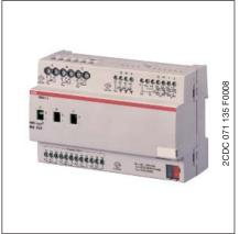
The Room Master Basic is a modular installation device (MDRC) in Pro*M* design. It is intended for installation in the distribution board on 35 mm mounting rails. The assignment of the physical address as well as the parameter settings is carried out with ETS 2 from version V1.3a or higher. The device is powered via the ABB i-bus<sup>®</sup> and does not require and additional auxiliary voltage supply.
